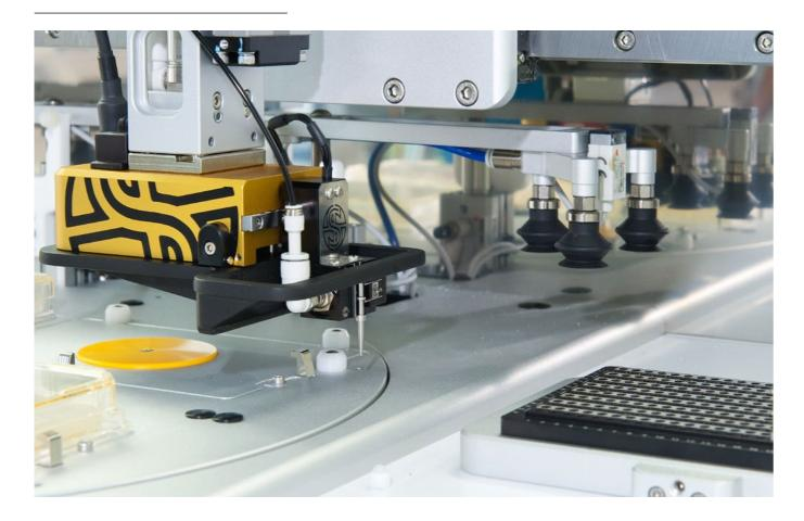
WHAT IS IT? The Stinger is an automated modular extension to the ROTOR HDA robot for easy, ultra-fast rearrangement of high-density library arrays of yeast, other fungi, bacteria, and algae from colonies grown on solid agar or in liquid culture. It is designed for the picking and spotting of user-specified colonies from high-density arrays onto solid agars in 96-, 384-, 1536-, and 6144-density format.
