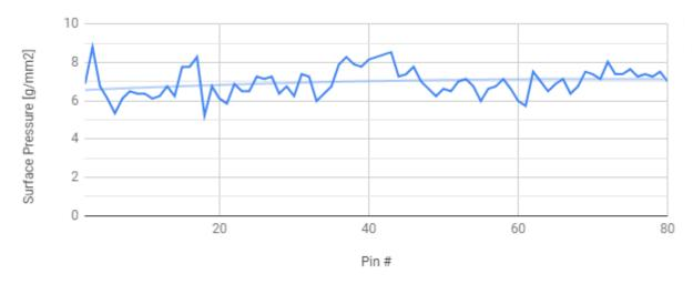
Each data point recorded is detailed below in Table 1. To account for the diameter of the PickupLine, a surface area of 0.785 mm<sup>2</sup> was used to calculate surface pressure.
