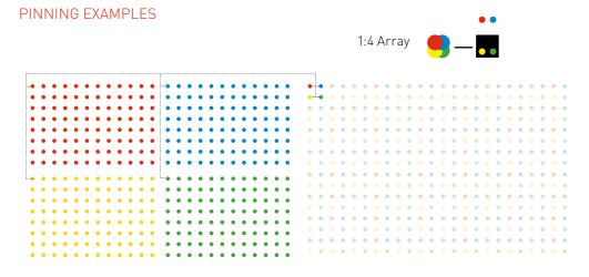
· 4x 96-density plates are combined onto 1x 384-density plate.
