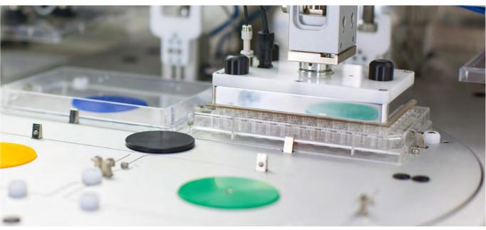
AGAR TO AGAR PINNING SPEED IS 25 SECONDS PER PLATE.
