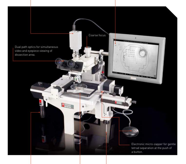
Joystick with X & Y stage control, fine focus and push-button software operation.
