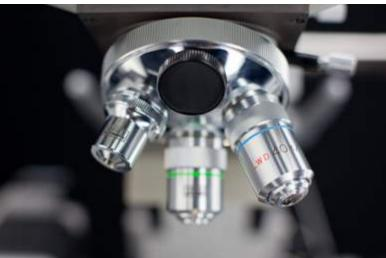
The special optics included are custom Singer x4 and THE x20 extra long working distance objectives and x15 OPTICS widefield eyepieces. The microscope has a daylightwhite 50,000 hr. LED light source with intensity control. Condenser illumination is via a special window in the sub-stage to minimise airborne contamination.
