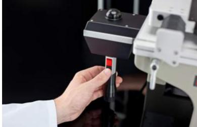
The comfortable joystick can control all the basic THE CONTROL functionality of the MSM 400. For two modes of X and JOYSTICK Y stage movement, two thumb-buttons and fingertip microscope focusing. The joystick and micromanipulator are located on opposite sides of the stage and can quickly and easily be configured for right or left-handed users.
